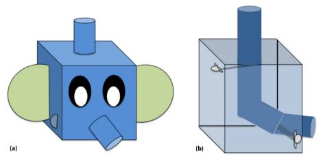
Figure 3. Schematic drawing of (a) exterior and (b) interior of Mr. Elephant apparatus with levers used by the experimenter to control the path of the balls through the tubes.
